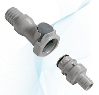
HFC12 Series couplings have flow comparable to many 1/2" flow couplings in a 3/8" body size. Compact and lightweight, HFC couplings replace bulky and heavy brass ball-and-sleeve couplings in a wide range of applications. An ergonomic design and a large, shrouded thumb latch pad produce a coupling that is easy to grip and simple to operate. An efficient valve design leads to high flow and low spillage.
