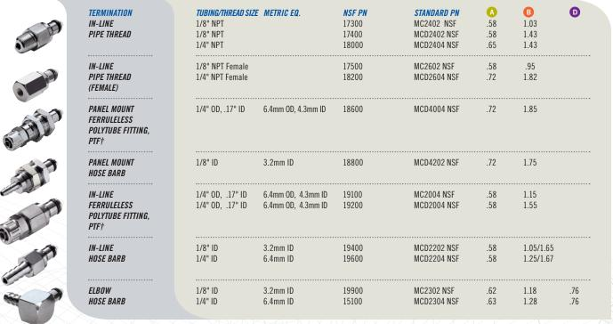
All measurements are in inches (millimeters) unless otherwise noted. Tubing must meet stated inside and outside diameters. †Note: CPC's Ferruleless PTF (polytube fitting) terminations do not require ferrules to achieve a secure connection and are therefore easier to use and reuse. PTF fittings are designed for semirigid tubing, i.e., polyethylene, nylon, polyurethane, etc.
