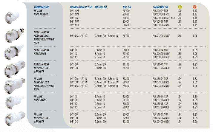
All measurements are in inches (millimeters) unless otherwise noted. Tubing must meet stated inside and outside diameters. †NOTE: CPC's Ferruleless Polytube Fitting terminations do not require ferrules to achieve a secure connection, which makes them easier to use and reuse. PTF fittings are designed for semi-rigid tubing, i.e., polyethylene, nylon, polyurethane, etc. NOTE: JG is a registered trademark of John Guest USA, Inc.
