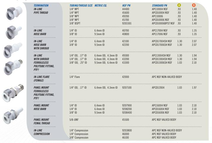
All measurements are in inches (millimeters) unless otherwise noted. Tubing must meet stated inside and outside diameters. †NOTE: CPC's Ferruleless Polytube Fitting terminations do not require ferrules to achieve a secure connection, which makes them easier to use and reuse. PTF fittings are designed for semi-rigid tubing, i.e., polyethylene, nylon, polyurethane, etc.
